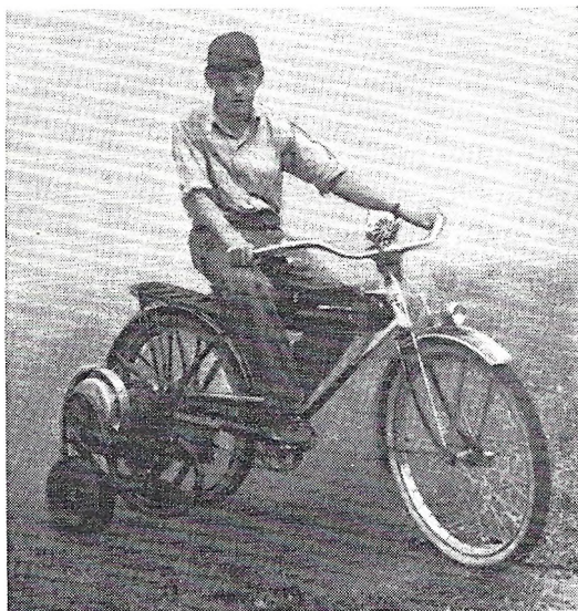
Morgan Ware converted his bicycle into a powered vehicle by adapting a washing machine motor to it as explained in MI.
