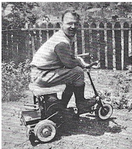
Built by John Mock, this scooter has three wheels instead of the usual two. It is powered by a washing machine motor.
