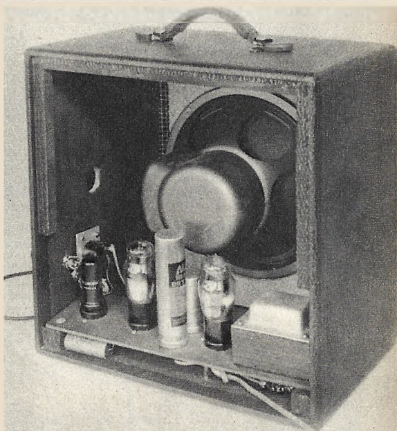
Above—A rear view of the amplifier showing the location of the parts. The power transformer is at the extreme right with the rectifier tube and filter condensers next. Below is the wiring diagram.
