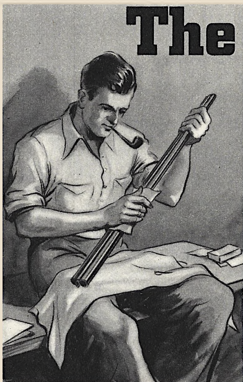
The final appearance of the metal parts will depend mainly upon the polishing done before the bluing.
