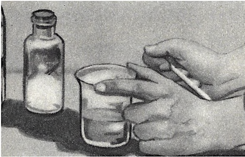
Nessler's reagent is used for testing for ammonia. When a few drops of this reagent are added to the water, a brown precipitate is formed if ammonia or salts of ammonia is present.
